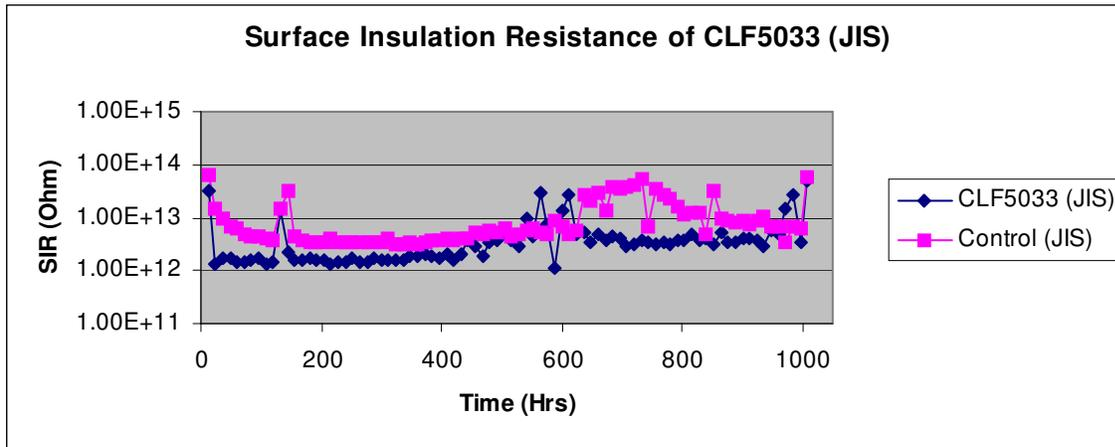
Surface Insulation Resistance:  $> 1.0 \times 10^{12} \Omega$ , passed.
