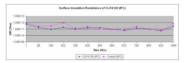
Surface Insulation Resistance:  $>1 \times 10^{10} \Omega$ , Pass.
