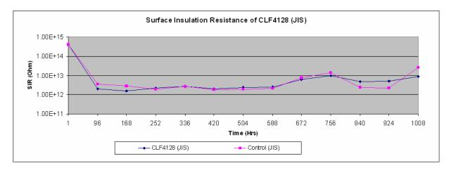
Surface Insulation Resistance:  $>1 \times 10^{12} \Omega$ , Pass.
