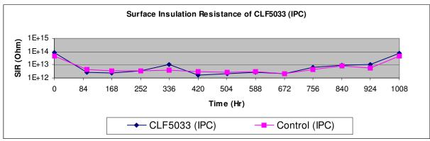
Surface Insulation Resistance:  $> 1.0 \times 10^{12} \Omega$ , passed.
