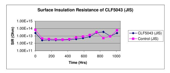
Surface Insulation Resistance:  $> 1.0x10^{12} \Omega$ , passed.
