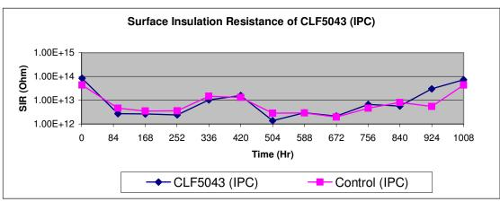
Surface Insulation Resistance:  $> 1.0x10^{12} \Omega$ , passed.
