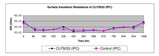
Surface Insulation Resistance:  $> 1.0 \times 10^{12} \Omega$ , passed.
